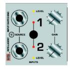
Using the Gain Knobs: The yellow LED for each channel should illuminate moderately under normal playing conditions with the gain knob about half way up
