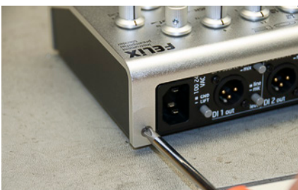
Fig.1 removing the chassis screws
